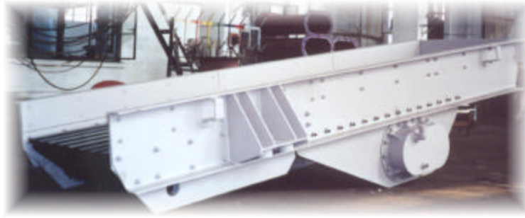
46" x 16' Vibrating Feeder After Assembly
